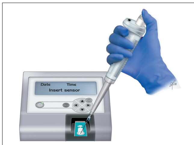
Figure 5.—A 30-μL semen sample is loaded on the sample port of the sensor strip.
