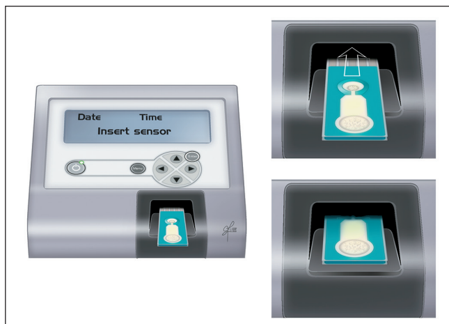
Figure 4.—The sensor should be placed on the port of the MiOXSYS® analyzer with the electrodes facing the analyzer. The sensor should be inserted by holding from side and the placing horizontal pressure on the sensor against the MiOXSYS® analyzer.
